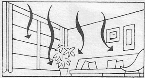
Ceiling cable is invisible. Wires less than \frac{3}{8} " thick are concealed within ceilings. Each room's temperature is individually controlled.
